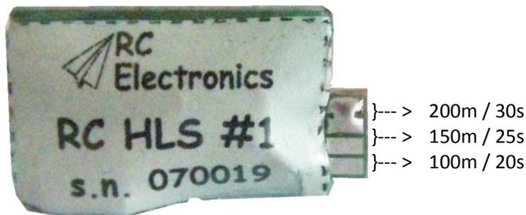
Figure 2: Soldering jumpers.
