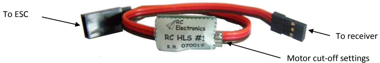
Figure 1: The RC HLS #1 module.
